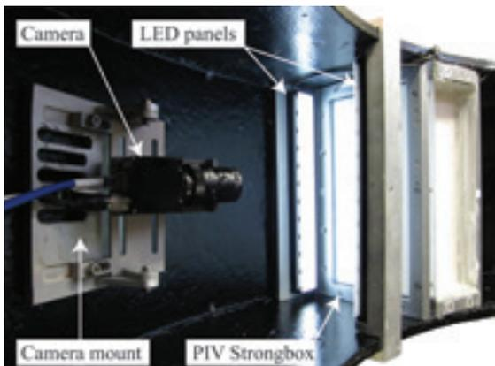
Figure 42: 'Next generation' PIV apparatus installed in the drum centrifuge channel
