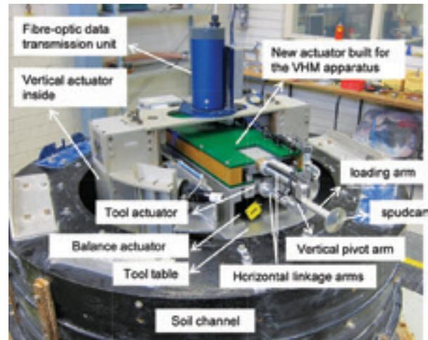
Figure 47: VHM loading apparatus for the UWA Drum Centrifuge
