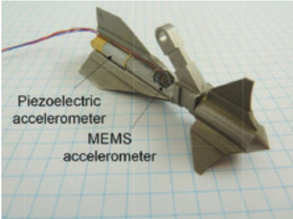
Figure 45: Accelerometers installed in a dynamically installed OMNI-Max anchor
