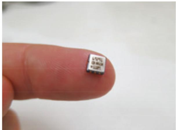
Figure 44: A  $\pm 500$  g MEMS accelerometer
