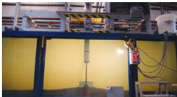
Figure 66: O-Tube test setup with large initial embedded pipe
