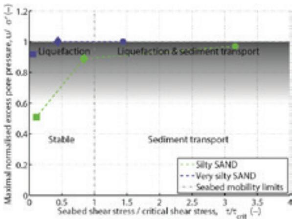
Figure 69. Seabed mobility matrix for typical NWS storms (square: <10 year storm, diamond: 10 year storm, circle: 100 year storm)
