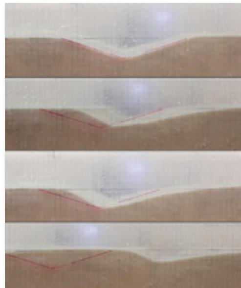
Figure 72: Model scale trench simulate din Mini O-Tube. The trench is migrating or 'running' to the left and become shallow and wide. Top to bottom, successive points in time
