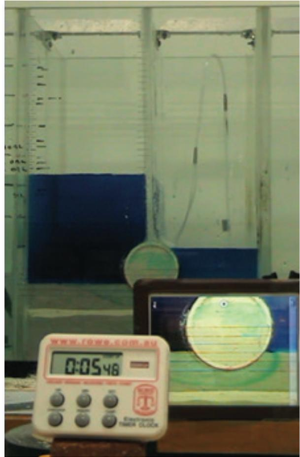
Figure 68: 'Fish tank' used to investigate piping beneath on-bottom pipelines. Fish tank background. In foreground is a close up video of seepage flow (in blue) beneath the pipe
