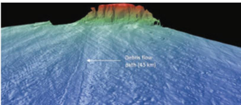
Figure 74: Seafloor rendering of Willem Survey showing large scale failure of the continental slope, small scale failures within the submarine canyons, and pock-marks indicating occurrence of fluid/gas expulsion in the mass transport deposit (inset). Sea-bed rendering developing using Seisnetics TM
