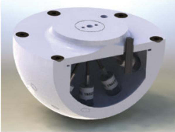
Figure 60: A CAD drawing of our hemispherical penetrometer for shallow seabed characterisation
