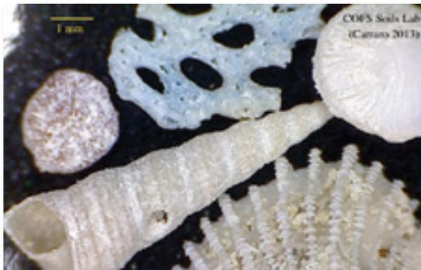
Figure 55: Typical particle shapes of carbonate sand used in the study
