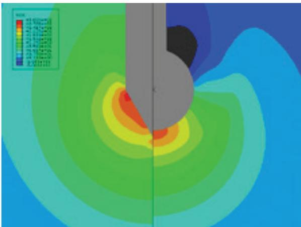
Figure 56: Excess pore pressure field around the ball and cone penetrometer
