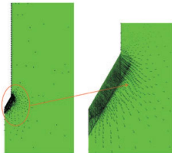
Figure 58: Flow mechanism of cone penetrometer
