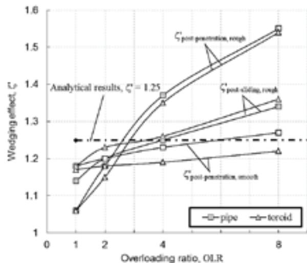
Figure 59: Wedging effect for toroid and ball ( $w/D = 0.4$ )
