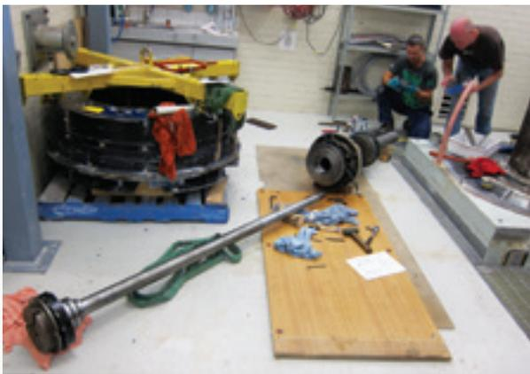
Figure 3: Rebuilding the drum centrifuge after the bearing replacement
