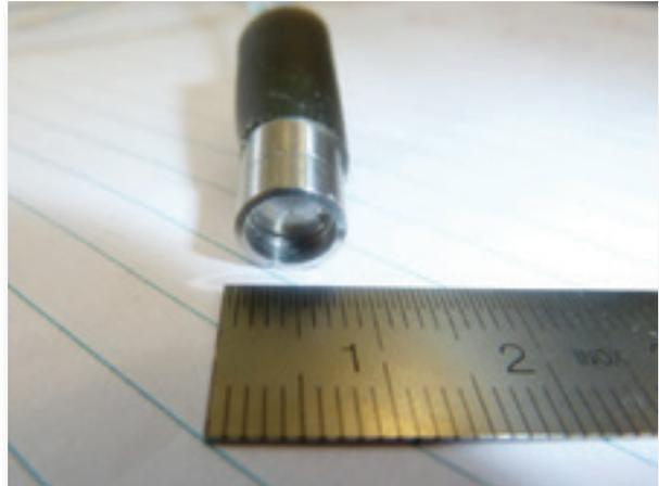
Figure 4: A prototype of the COFS new miniature pore pressure sensor
