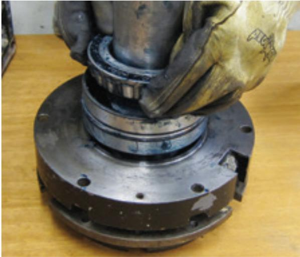
Figure 2: Installing the new preloaded roller bearing
