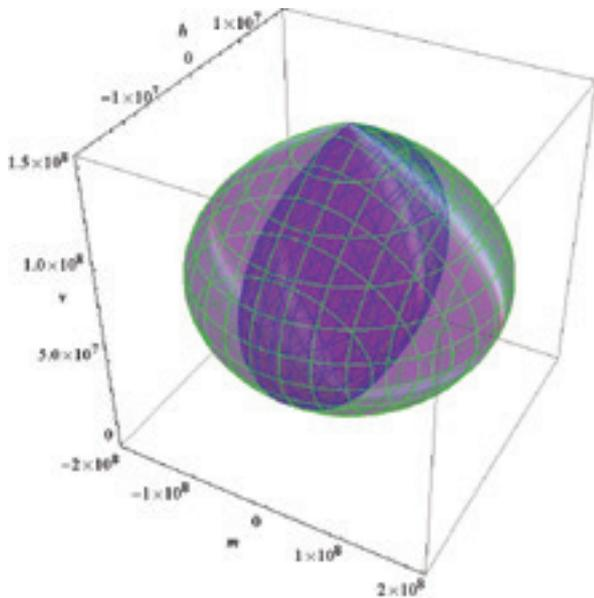
Figure 53: VHM yielding and bounding surfaces of a sample Jack-up foundation
