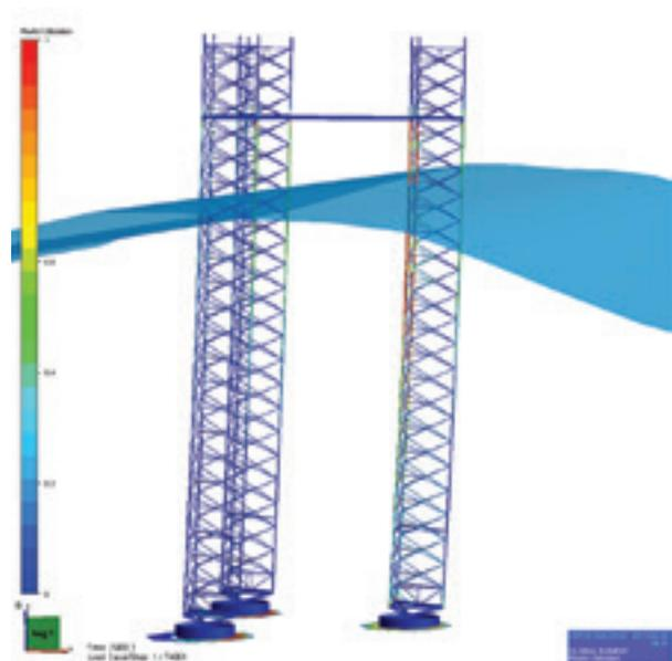
Figure 52: Typical structural collapse of a sample jack-up platform
