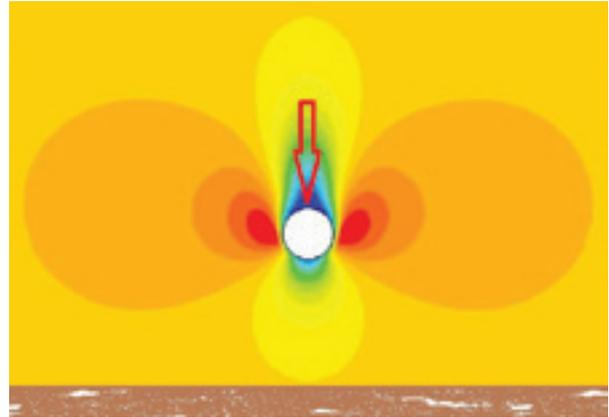
Figure 113: Contours of water particle velocities around an oscillating riser
