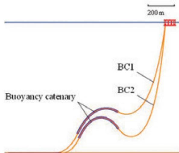
Figure 109: Illustration of the LWR configurations (superimposed view)
