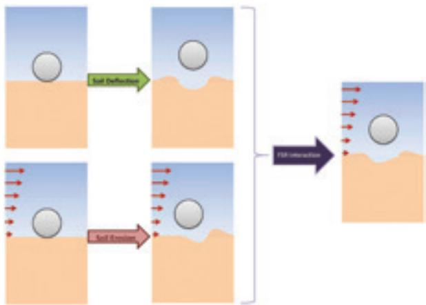
Figure 114: Merging soil deflection and soil erosion UDFs in FSR interaction
