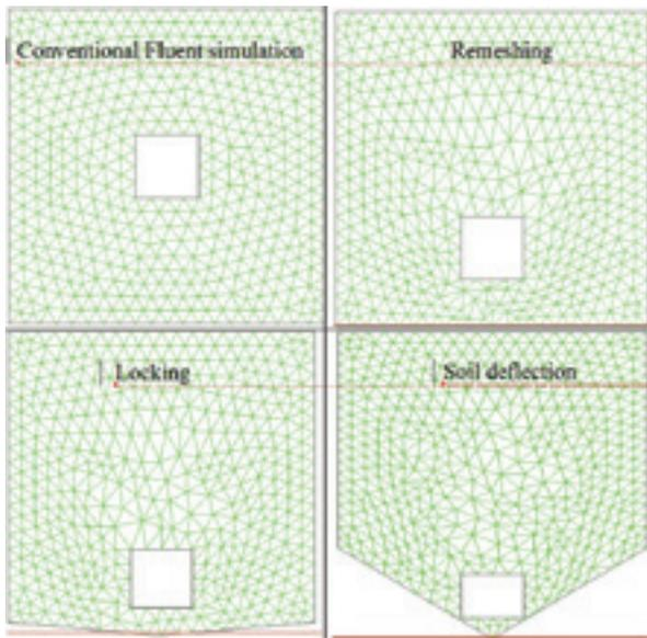
Figure 112: Schematic views for FLUENT simulation in FSR interaction
