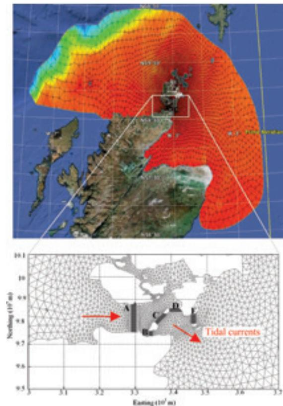
Figure 115: Map of the Pentland Firth, UK. Colour shading at top indicates bathymetry (i.e. water depth). Below, sections A through E indicate locations where tidal energy extraction has been modelled
