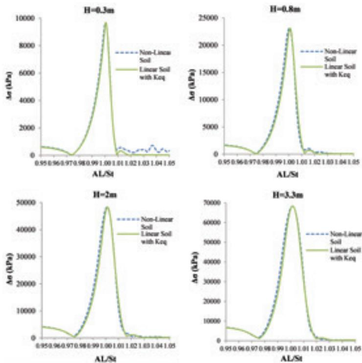
Figure 111: Comparison of the stress range distributions around TDP between nonlinear and equivalent linear soil models
