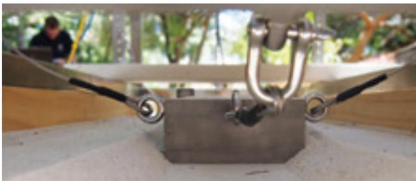
Figure 22: Close up of flat plate tool during a drag test.
