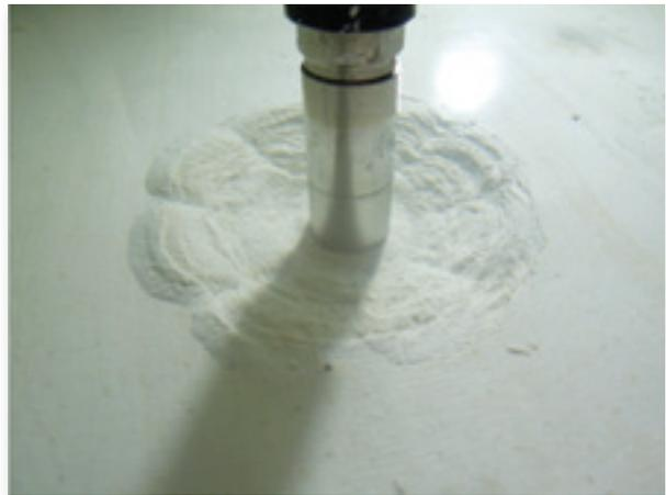
Figure 15: Evidence of soil expulsion through side openings and soil flow around (on top of spudcan)
