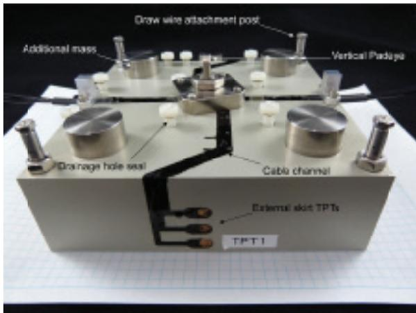
Figure 19: The model skirted foundation with its instrumentation
