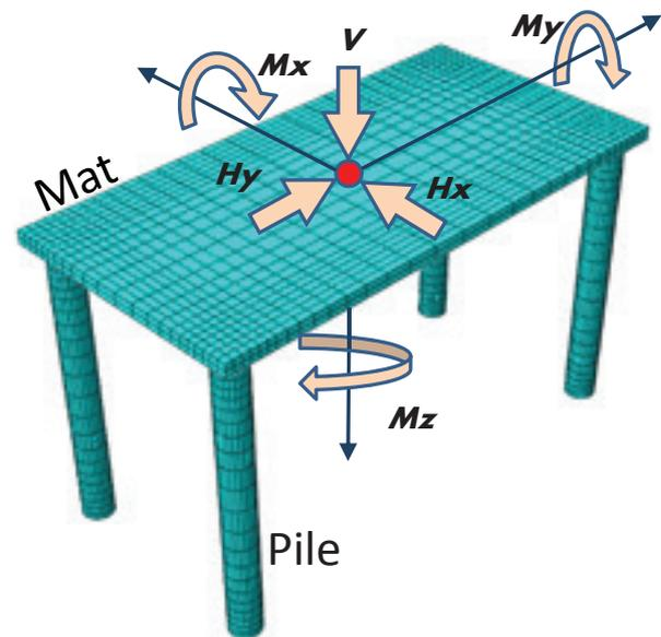
Figure 20: Configuration and loading conditions for hybrid subsea foundation (HSF)
