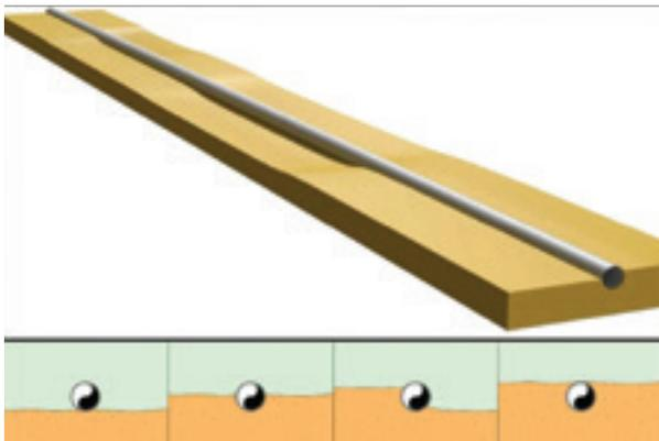
Figure 23: A reconstruction of the burial state of the 1TL pipeline (Jas et al. 2013)
