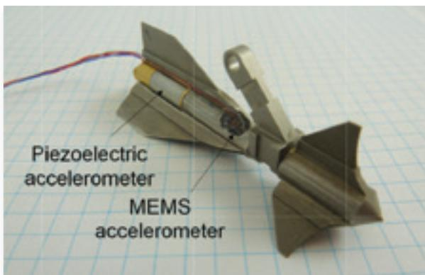
Figure 16: The Model OMNI-Max anchor featuring innovative accelerometer systems to measure both the deceleration of the anchor in the soil and its trajectory during pulling out
