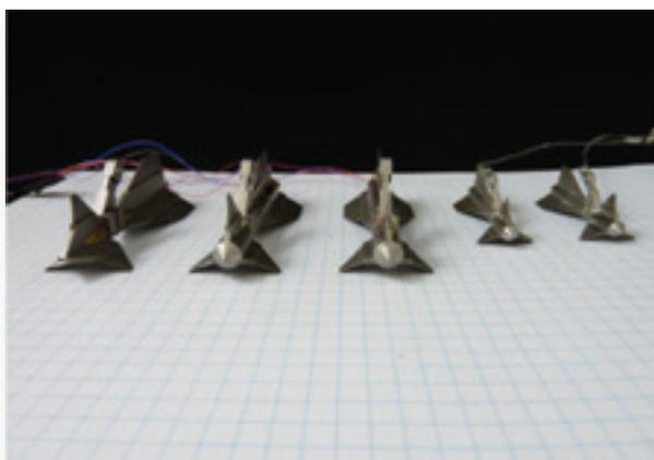
Figure 17: The five OMNI-Max model anchor featuring various amount of ballast and instrumentation
