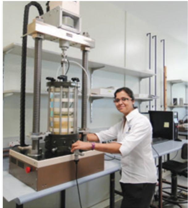
Figure 5: New 10-Hz Dynamic Triaxial apparatus being operated by Senior Soil Technician Usha Mani
