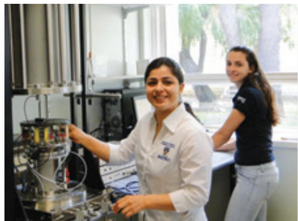
Figure 6: Senior Soil Technician Behnaz Abdollahzadeh and CNPq Fellow Marina Bortolotto setting up the new state-of-the-art 3-MPa Resonant Column apparatus at COFS
